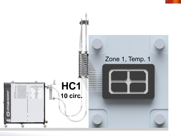
Circuit 1, flow rate 25 l/min
